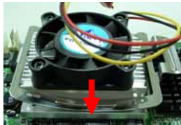
3. Put the cooler through the four pills on the base
