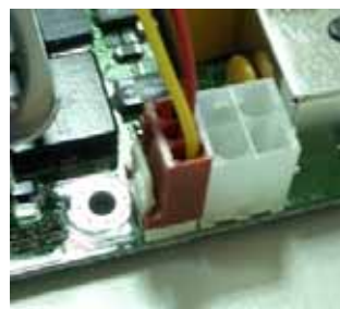
4. Connect the fan connector on CPU_FAN
