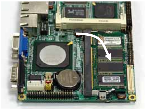
(2. Press down the module with a click sound)
